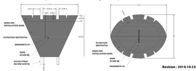
Drawing not to scale. During processing, the dimensions may vary slightly.
