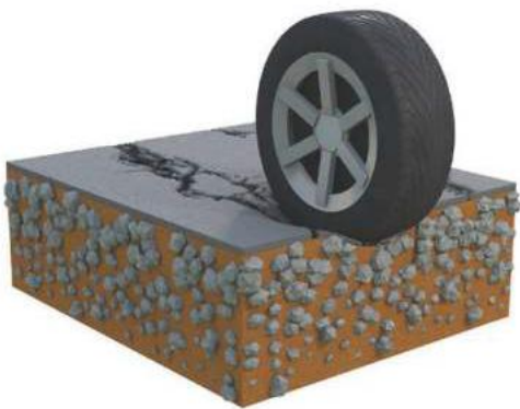
Figure 4 – Road structure without geotextile
