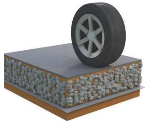
Figure 5 – Road structure with geotextile
