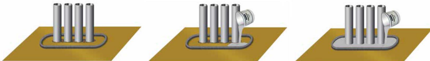
Figure 5: Closing several perforations with epoxy resin
