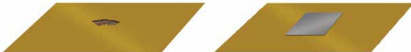
Figure 6: Repairing holes in the TM520 VBP
