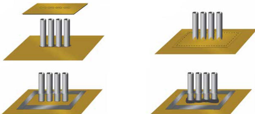
Figure 4: Closing several perforations with a piece of TM520 VBP
